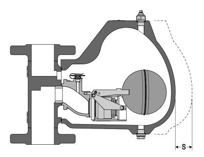
To remove the cover a withdrawal space S of 270 mm is required.
