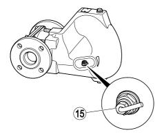
If you cannot prevent the stuffing-box packing from leaking fluid replace the whole float-lifting lever.
