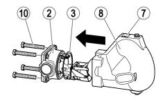
➤ If necessary, mount the measuring electrode as described on page 16.
